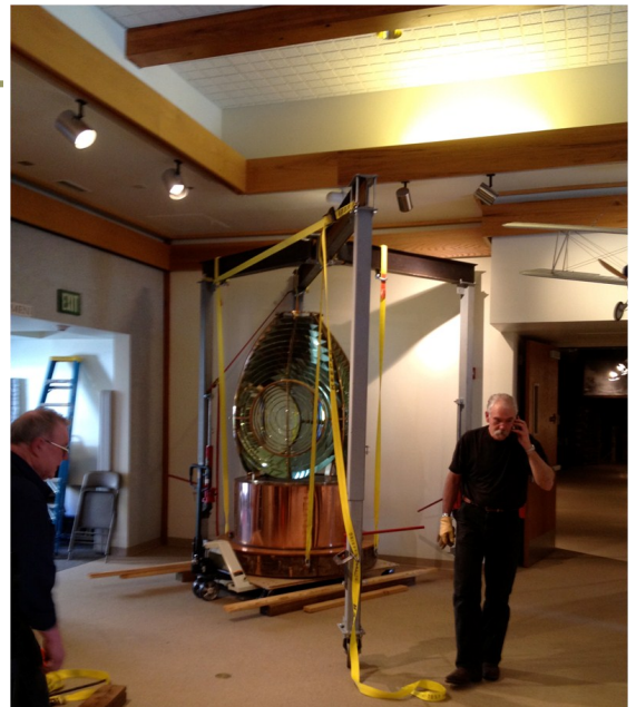
Crane wrapped around the lens and ready to be lowered onto the modified pallet jack. Bob multi-tasking while Tom looks on.
